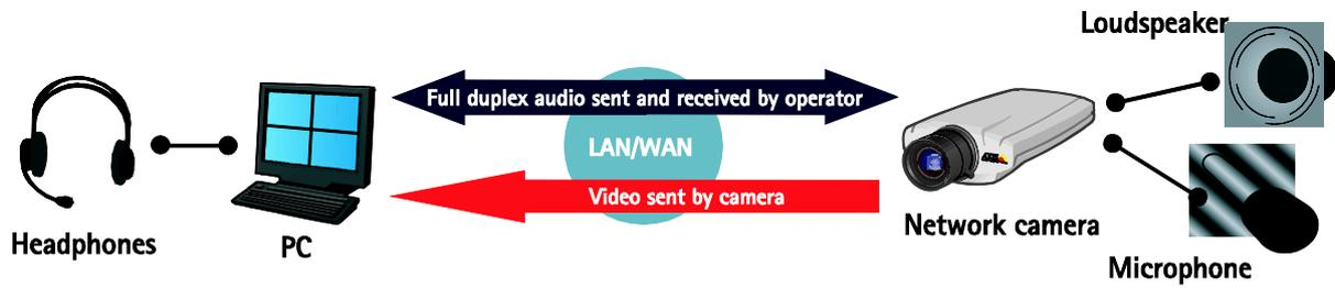
**Figure 6.4** Full-duplex mode. Full-duplex mode is similar to a telephone conversation.
