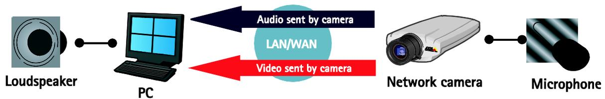
**Figure 6.1** Simplex – Microphone only mode. Audio is transmitted from the camera/video encoder to one or more clients. Applications include remote monitoring, web attractions, etc.
