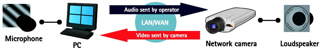
**Figure 6.2** Simplex – Speaker only mode. Audio is transmitted from a client to the network camera and played by a speaker connected to the camera. To send audio from the client, the Talk and Microphone buttons in the AMC toolbar (see 5.1.2) must both be enabled.
