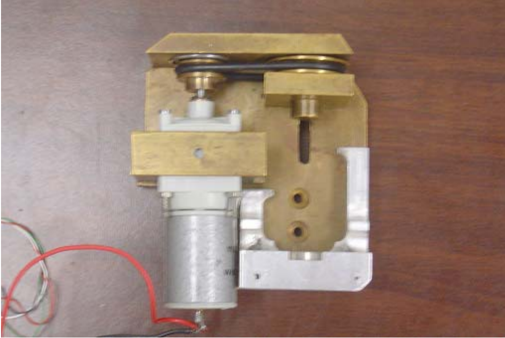
Figure 4-4. Testing Device used by Mindess & Diamond (1980) for SEM testing on cement mortar
