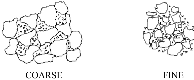
Figure 2-6. Aggregate Structure for Coarse and Fine Mixtures (Nukunya et al. [2001])
