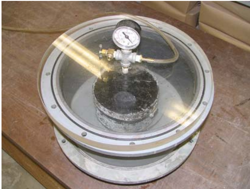
Figure 6-4. Vacuum Saturation of sample prior to moisture conditioning
