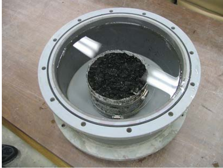
Figure 6-3. Compacted pill rolled in 1/8" inch sample placed in vacuum chamber
