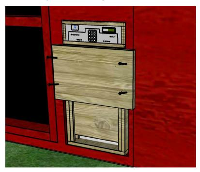
If you need to close off any open area above Coop Tender, simply cut an appropriate size piece of wood or other suitable, predator proof, material and secure it.
