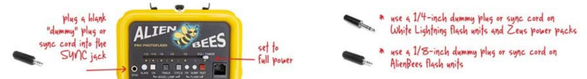
**7. Insert a dummy plug in the sync jack of each flash unit or power pack.** The dummy plug will disable the slave eye, preventing the flash from being tripped and fired whenever the flash of light from another unit is detected. **Note:** To disable the sync jack, you can insert a dummy plug (sold separately on our website) or plug in the sync cord that came with the flash unit or remote, plugging in the 1/8-inch or 1/4-inch sync jack end only.
