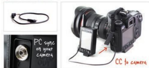
**Sync Cord Connection:** Cameras with an absent or occupied hot shoe can be hardwire connected using the provided SC-CST sync cord. The cord plugs into the 2.5mm sync jack located on the left side of the Cyber Commander™ unit and into the camera's PC sync (flash terminal) connection.
