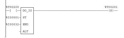
The example DO I/O function block above will update both the bit and word data for a module with a %I starting reference of %I00001. When the DO I/O function receives power flow and output references are specified, the output points starting at the reference ST and ending at END are written to the referenced module(s).
