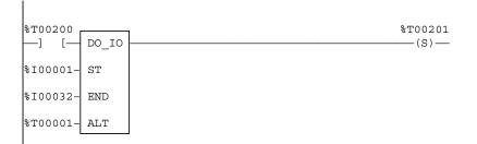
If previous outputs have not been consumed because DO I/O has been attempted within less than one module sweep since outputs were last written, then DO I/O terminates and does not pass power flow.
