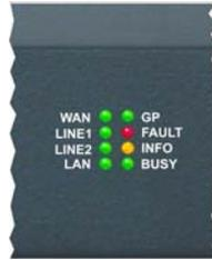
Fig. I-4: QuadroM-E1/T1's Front Panel LEDs
