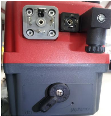
Figure 13 – Small connector removed
