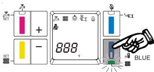
You can adjust the DHW draw-off temperature by keeping the PURPLE "**B**" key pressed down, and simultaneously pressing the keys "+" to increase the temperature or "-" to reduce it.
