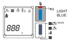
it will display the boiler's error code, in place of the temperature "U", after the fault indicating led "R" has illuminated.
