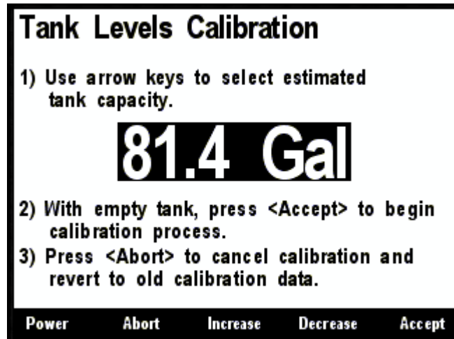
Figure 213 – Tank Levels Calibration Capacity Estimation
