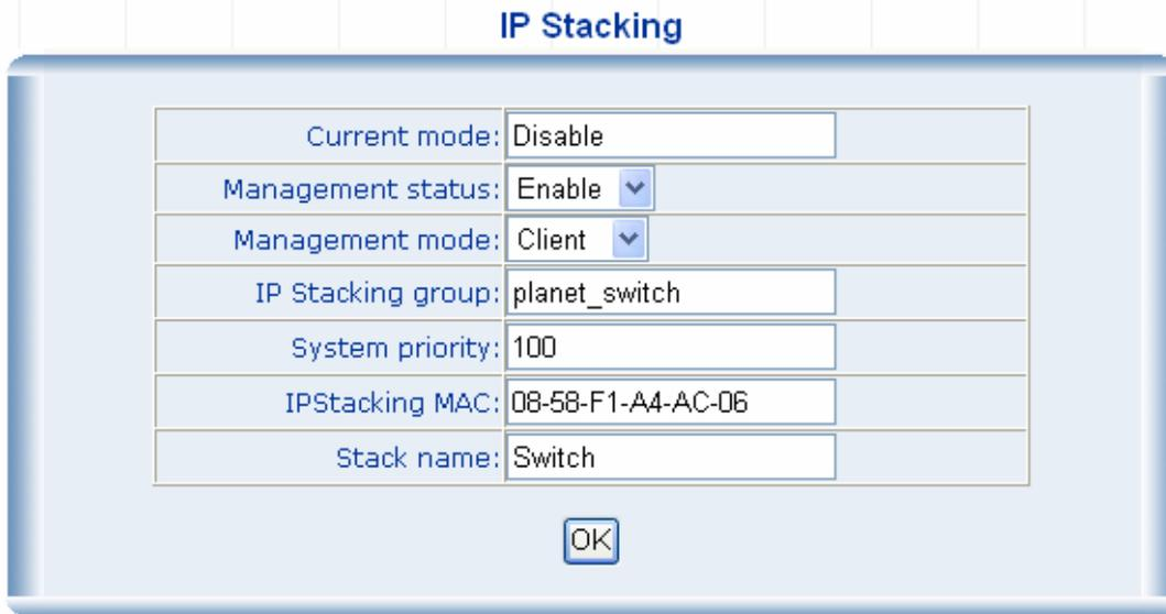
9. Modify the **“System priority”** and **“Stack name”** if necessary. At this sample we change the Stack name of the Client to “Switch-2”
