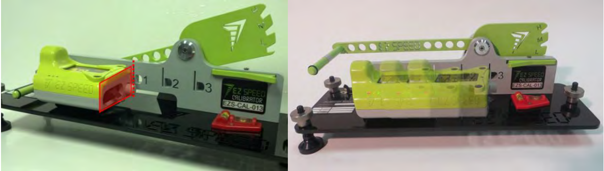
Figure 4: Positioning for D1 (left) and 3 Positions of EZSpeed on Calibrator (right)
