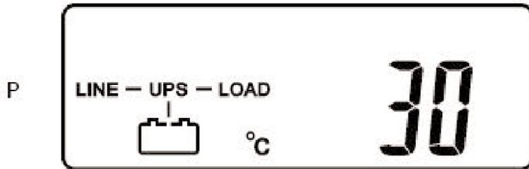
The degree C symbol indicates the reading is for the internal UPS temperature.
