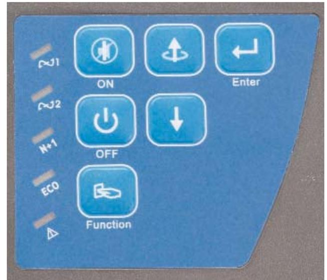
2. When the LCD is in the “Display Programmed Settings” mode, depressing the Function Button will return the LCD to normal mode. The LCD display will also return to “Normal Mode” automatically after 30 seconds of button inactivity.
