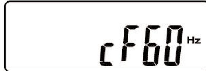
Setting the UPS to a fixed or constant output frequency should be done when the input source is a generator.
