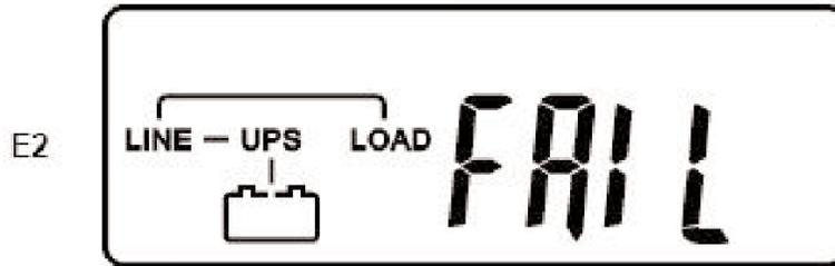
If the UPS fails the self-test, "FAIL" is displayed alternately with an error code. Please note the error code and contact Falcon Service.
