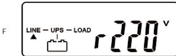
The UPS is now turned on and in on-line inverter mode. Using an AC volt meter, verify the UPS input voltage measurement.
