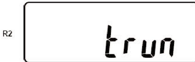
If the “Previous Page/Change Setting” button is pressed, a UPS self-test will be initiated and the following displays will be shown.
