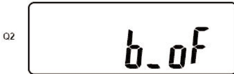
If the “Previous Page/Change Setting” button is pressed, the audible alarm will be turned off. Depressing the button again will turn the alarm back on. Depress the “Next Page” button.
