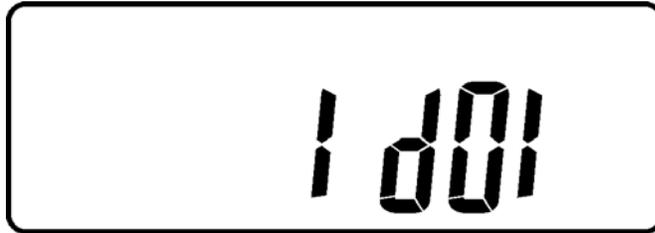
The next parameter displayed shows the UPS unit address. If only one UPS is being used, the address should be set to “d0” as shown.
