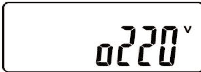
The next parameter display is the inverter output voltage setting. The inverter output voltage can be set to 200Vac (not shown), 208 OR 220Vac (shown), 230Vac (not shown) or 240Vac (not shown).
