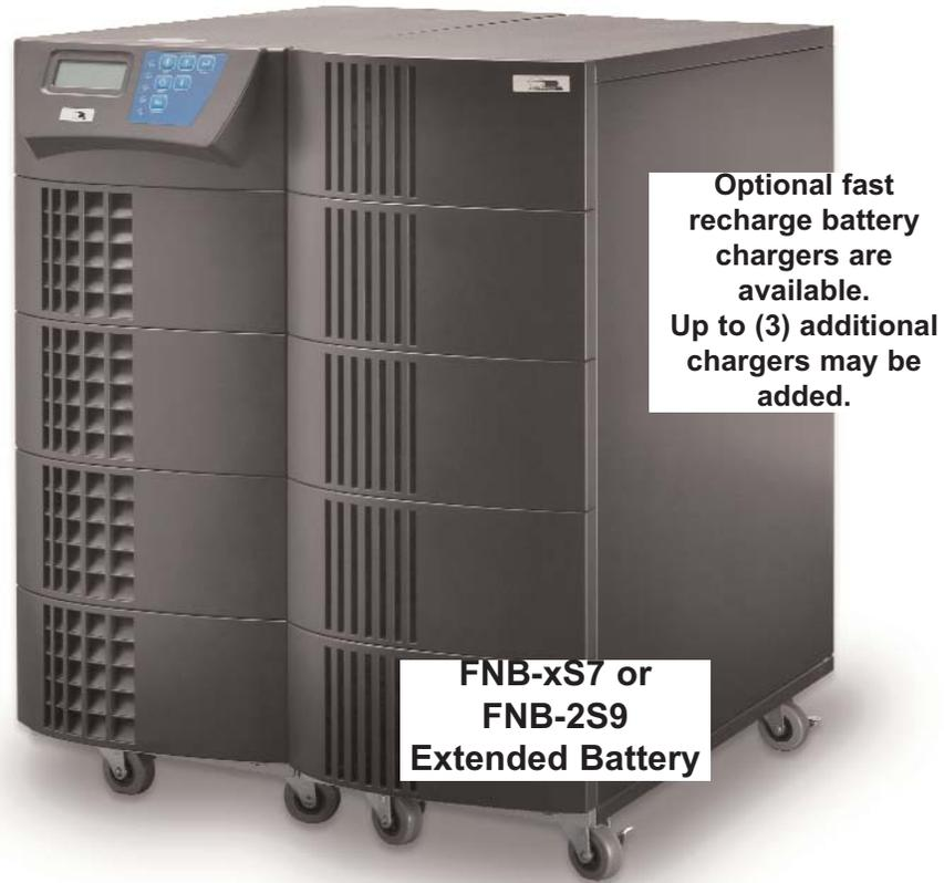
FN Series Extended Battery Bank Option contains: one, two or three 240Vdc parallel strings of 12V, 7AH, Valve Regulated Lead Acid (VRLA) batteries depending on the model. The FNB-1S7 model adds one additional battery string, the FNB-2S7 adds two, and the FNB-3S7 adds three. All strings are in a single battery bank enclosure. Multiple enclosures may also be configured. When connected to the FN -2TXI model UPS, the Extended Battery Bank will provide an extended battery backup time.
