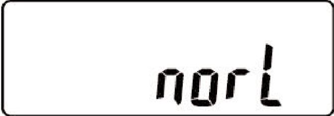
The following V1, V2, V3 and V4 show the operational status setting of the UPS. This function may be set to one of four modes. "Normal": which indicates none of the other modes are set.
