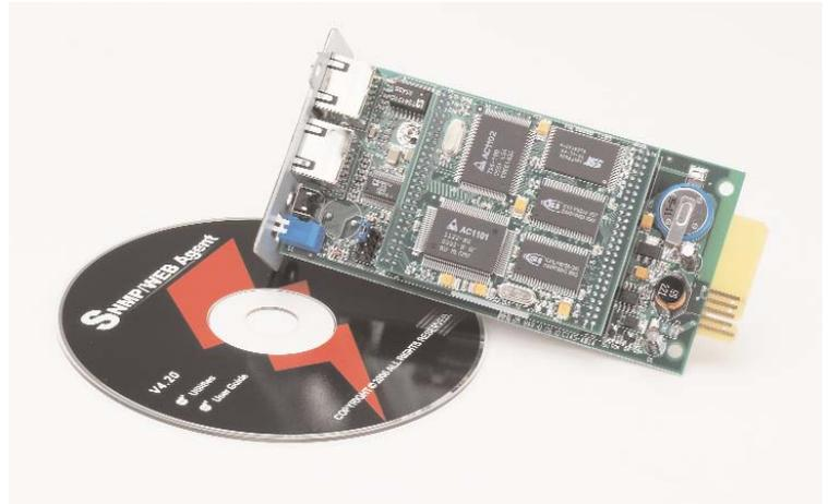
Remote server and computer shutdown client software is also provided. The software supports the shutdown of multiple servers or computers "in-band" across any Ethernet LAN. The client software may be installed on as many systems as required and supports most MS Windows and server platforms, in addition to LINUX.
