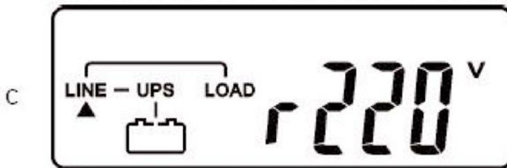
Note the MIMIC portion of the display with the arrow under the line and the input voltage is displayed.
