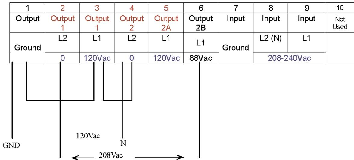
The 120Vac output must never be loaded more than 50% of UPS output rating.
