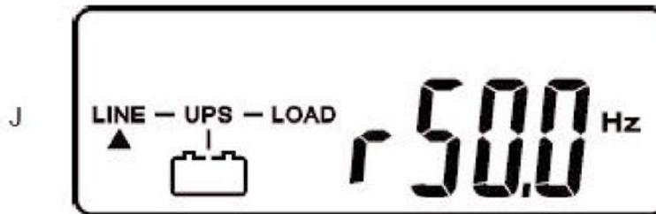
The "r" denotes the reading is for utility. The arrow under the LINE indicates the reading is for the utility frequency.
