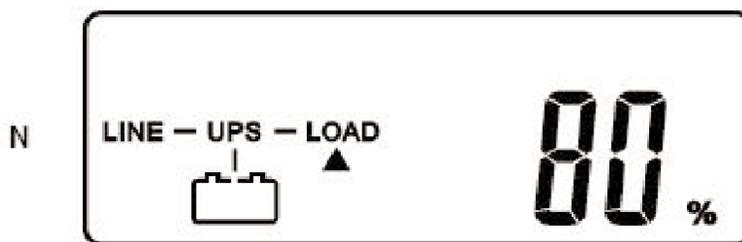
The arrow under the LOAD indicates the reading is for the UPS output and indicates the percentage of output load connected to the UPS.
