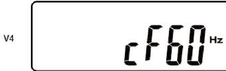
Setting the UPS to a fixed or constant output frequency should be done when the input source is a generator.
