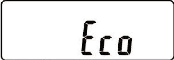
The Economy/Green Mode: indicates the UPS will automatically transfer to bypass mode to save energy, should the output load drop below 10% of the UPS output rating.
