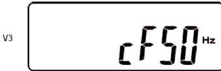
Fixed or constant frequency output mode: In normal mode the UPS output frequency will automatically be set to the utility frequency and is synchronized with that frequency. When set to cf50Hz mode, the UPS inverter output frequency will always be 50Hz. When set to cf60Hz mode, the UPS inverter output frequency will always be 60Hz.
