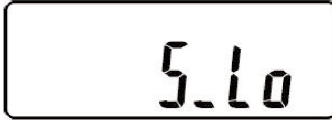
The next parameter displayed shows the “bypass input voltage acceptable window” setting. The voltage window can be set to “Lo” (184-260Vac) or “Hi” (195-260Vac), which is shown below.
