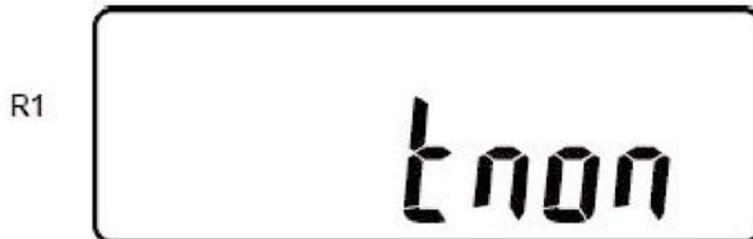
Next, the self-test status is displayed. Here the self-test is shown to be in the “Test Not On” state.
