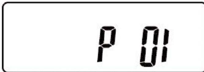
The next parameter displayed defines when the UPS is used in a parallel configuration. The settings are “P01” and “P02”, If only one UPS is being configured (not paralleled), the position should be set to “P01” as shown. If UPS units are connected in parallel it should be set to P02.
