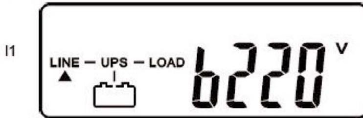
The "b" denotes the reading is for the bypass. The arrow under the LINE indicates the reading is for the bypass input voltage.
