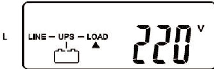
The arrow under the LOAD indicates the reading is for the UPS output voltage.
