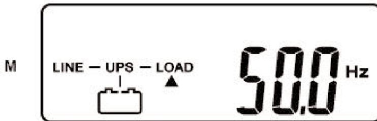
The arrow under the LOAD indicates the reading is for the UPS output frequency.
