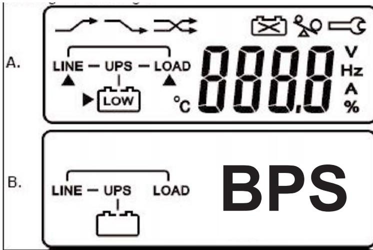
Display A is an LCD test display and is shown for about 3 seconds after the input circuit breaker is turned on.
