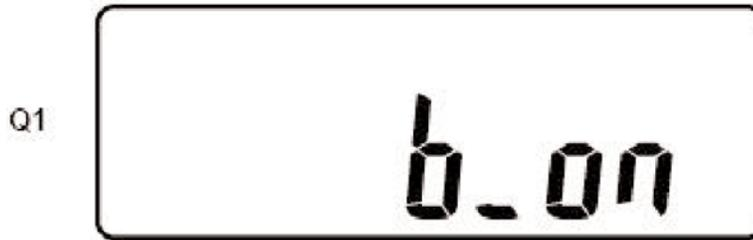
The first function status displayed will be the audible alarm buzzer status. It is shown here to be turned on.
