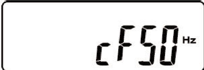
Fixed or constant frequency output mode: In normal mode the UPS output frequency will automatically be set to the utility frequency and is synchronized with that frequency. When set to cf50Hz mode, the UPS inverter output frequency will always be 50Hz. When set to cf60Hz mode, the UPS inverter output frequency will always be 60Hz.
