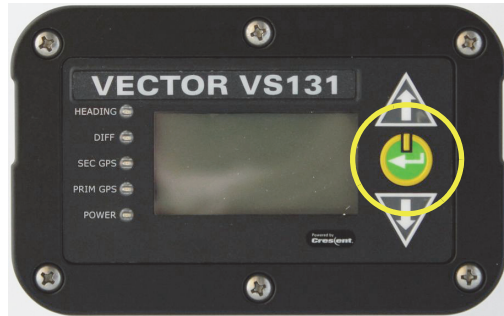
Figure 4-1: VS131 front panel with power button
