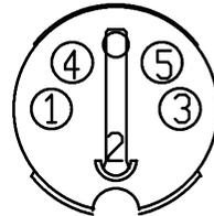
5-pin DIN-connector at TNC
