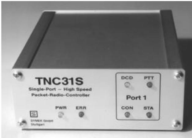
TNC31S: Single port controller up to 1 Mbit/s. 128 or 512 Kbytes Flash-EPROM, max. 512 Kbytes CMOS-RAM. Software same as TNC3S.
