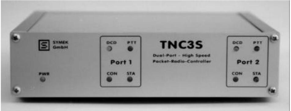
TNC3S: Dual port packet-controller (two independent modems), 256 Kbytes Flash-EPROM, max. 2 Mbytes CMOS-RAM, max. 1,6 Mbit/s total data rate. Software: Hostmode, Mailbox, KISS, SLIP, Hayes, Sixpack, X-Net.
