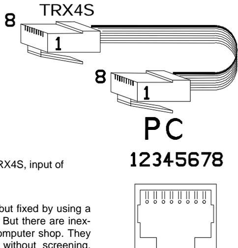
*RJ-Connector, rear view.
