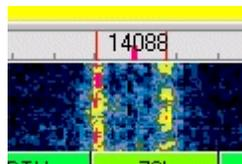
Figure 4. RTTY signal's two vertical lines.
