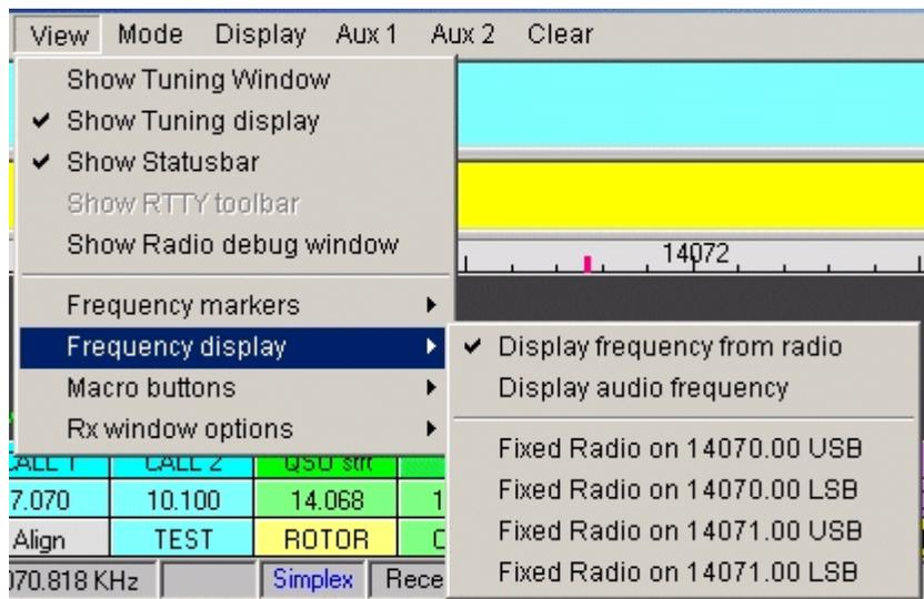
Logger32 can display a maximum of 4000 Hz. of receive bandwidth (receive range), however, it will only receive and transmit over 3000 Hz. bandwidth, from 0 Hz. to 3000 Hz. of audio.
