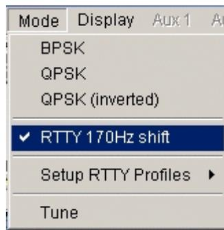
Figure 2. RTTY selected from the drop-down menu.
