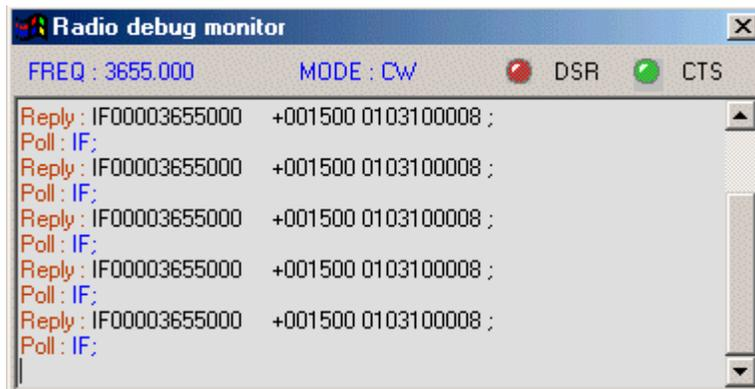
This window monitors the serial link between Logger32 and the radio and displays:
