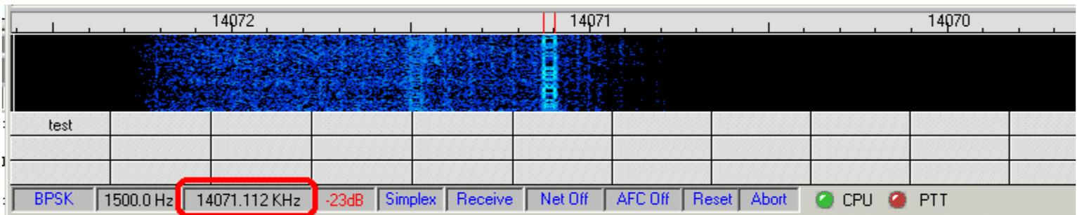
**Note:** Logger32 may or may not reflect a change in frequency that you set using your RIT or clarifier control on the radio. You should check this so you know how it works. Turn the RIT or clarifier and see if the frequency pane shows a change.
