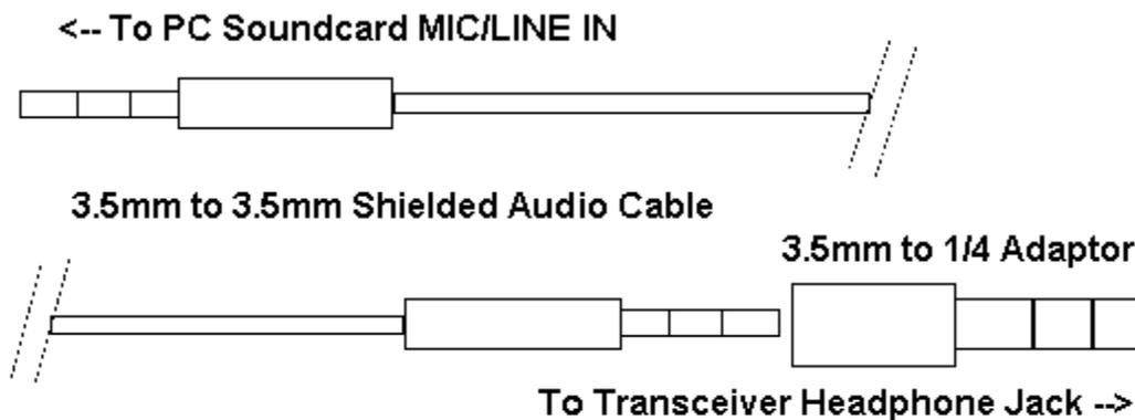
In some setups, with the headphone jack part of the way in, you can monitor transceiver audio through the radio speaker while sending the audio to the sound card. This is a great aid in tuning signals by ear while monitoring them on Logger32's tuning
