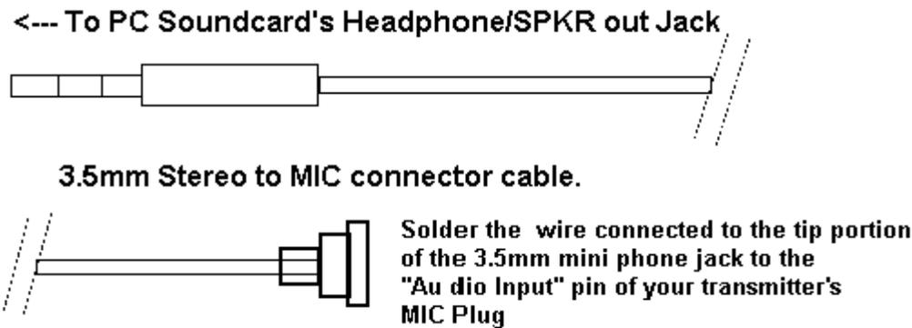
With the above interface connected, and your transceiver's antenna jack connected to a dummy load, set the audio output level of your PC sound card to match your transceiver's input circuit.
