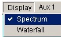
In Waterfall mode, if the background turns red then the sound card input level is too high. In the Spectrum mode, the entire spectrum line will turn red in this situation.
