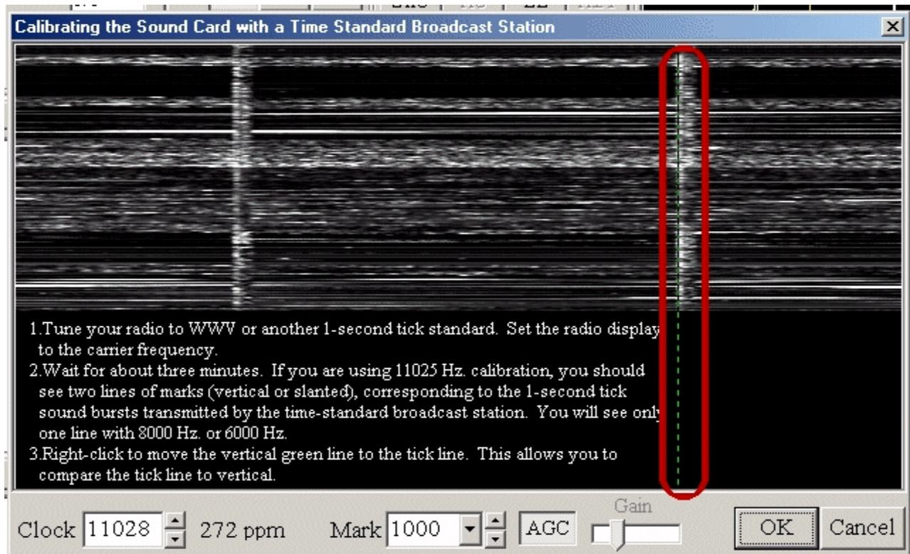
Here are two pictures of Russian time standard station RWM. The first shows a properly adjusted display. The second illustrates error of 1000 ppm. Note the slanted lines. This will occur with any time standard if you have an error of 1000 ppm.
