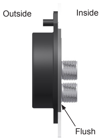
Figure 18: Entry Seal with Housing Installed
