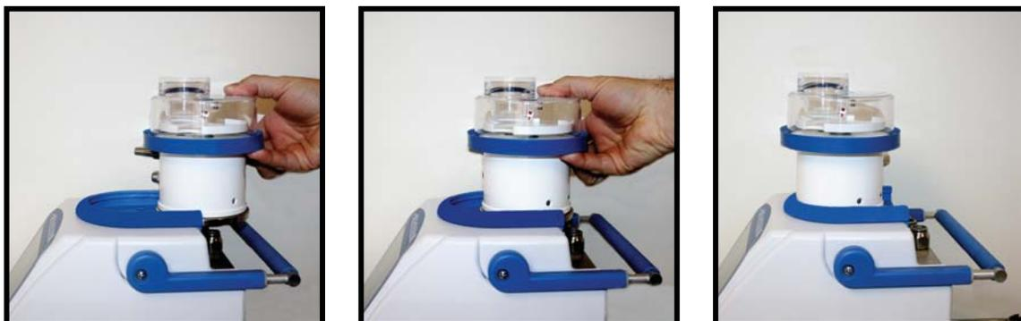
Once secure within the transport cup, the transport handle can be extended and raised to a position above the sampler. Use the handle to transport the V100 and R2S/RCG sampler to the desired location. Once in the desired location, the handle can be returned to the rear of the V100 and collapsed into its storage position. When removing the samplers, ensure that the handle is out of the path of the sampler, lift the sampler up slightly and slide to the rear of the transport cup.
