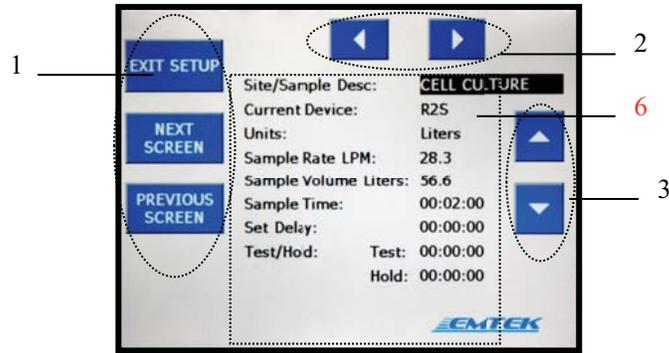
Fig 7.2.2 Setup Screen 2 Sample and Test Information
