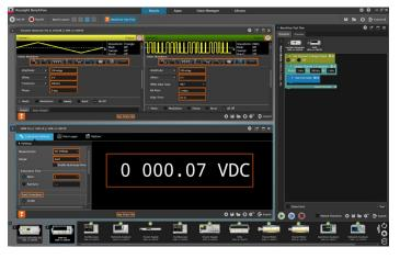
BenchVue Test Flow is integrated into the BenchVue framework and occupies the right-hand panel of the user interface.
