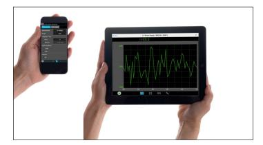
**BenchVue mobile** is a mobile app that you can install on an Android or Apple iOS device to control BenchVue bench applications running on your Windows computer. BenchVue mobile connects to your computer as a client, and requires that your mobile device and computer be connected to the same local network or intranet (behind the same corporate firewall). This network connection can be made via a WiFi connection inside your work location or externally through a VPN connection.
