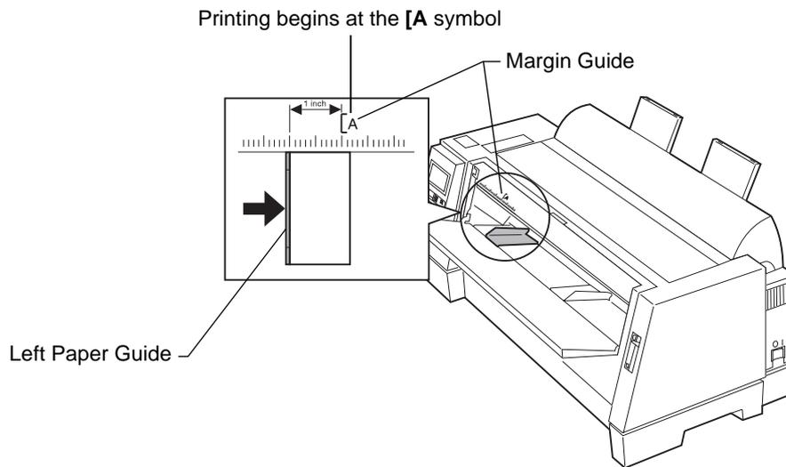
The distance from the left paper guide to the [A] symbol determines the width of the left margin.
