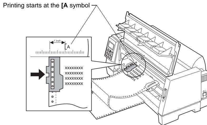
The distance from the [A] symbol to the left edge of the paper determines the width of the left margin.
