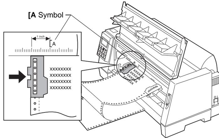
Pull up the left and right tractor locking levers to unlock the tractors.
