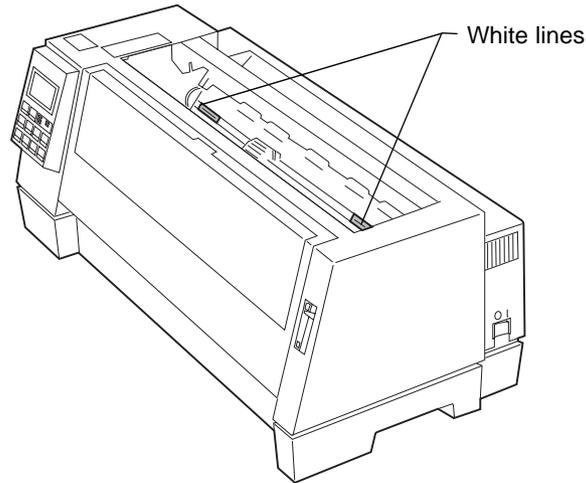
**Note:** When the ribbon cartridge is installed and the top edge of the paper is even with the top edge of the ribbon, the TOF is set to one line, or 1/6 inch.
