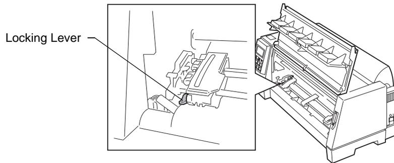
Move the left tractor to the left or right of the [A symbol. Push down the left tractor locking lever to lock it in place. Remove slack from the paper and lock the right lever.
