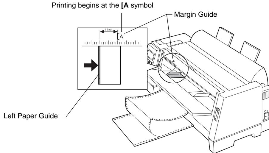
The distance from the left paper guide to the [A] symbol determines the width of the left margin.
