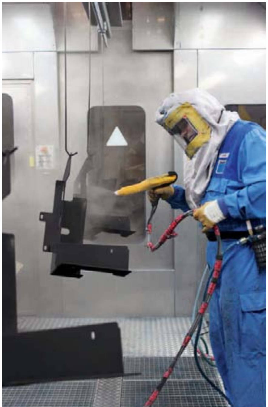
After selecting the program for parts that are difficult to coat: “The powder moves easily into the corners and the edges. There is no powder build-up in the corners.”
