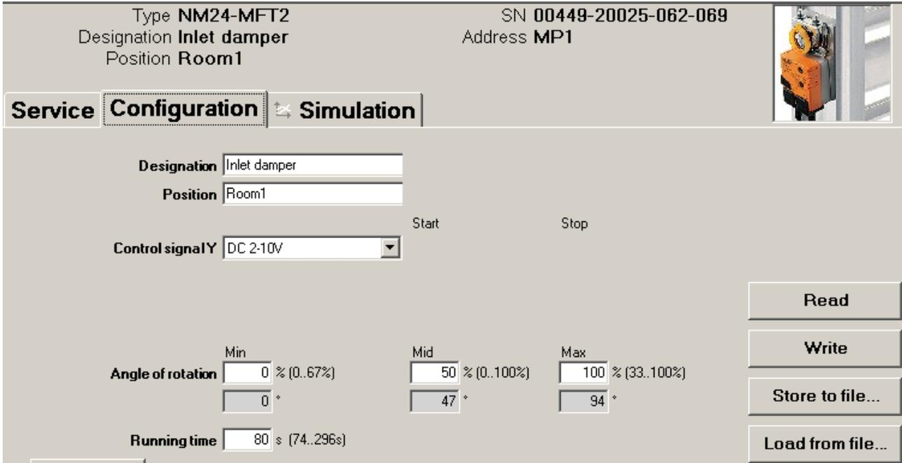
Example of the "Configuration" tab (damper actuator)
