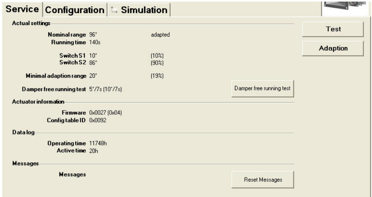
"Service" tab for BF-TopLine fire damper actuators
