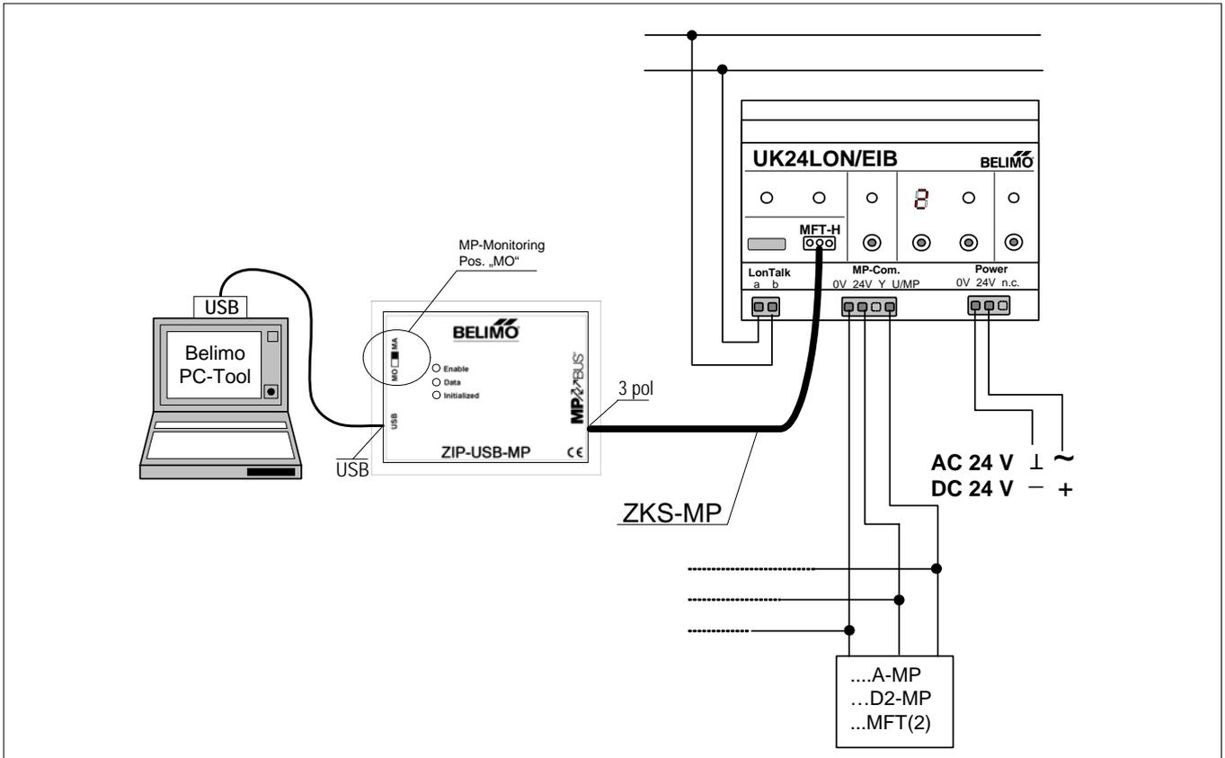
Typical wiring diagram 6
