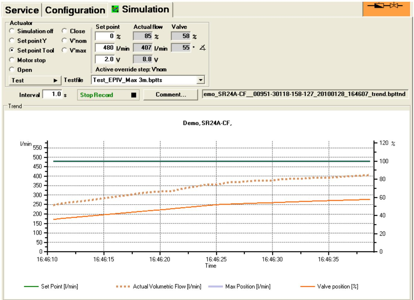
"Simulation" tab for VAV controllers
