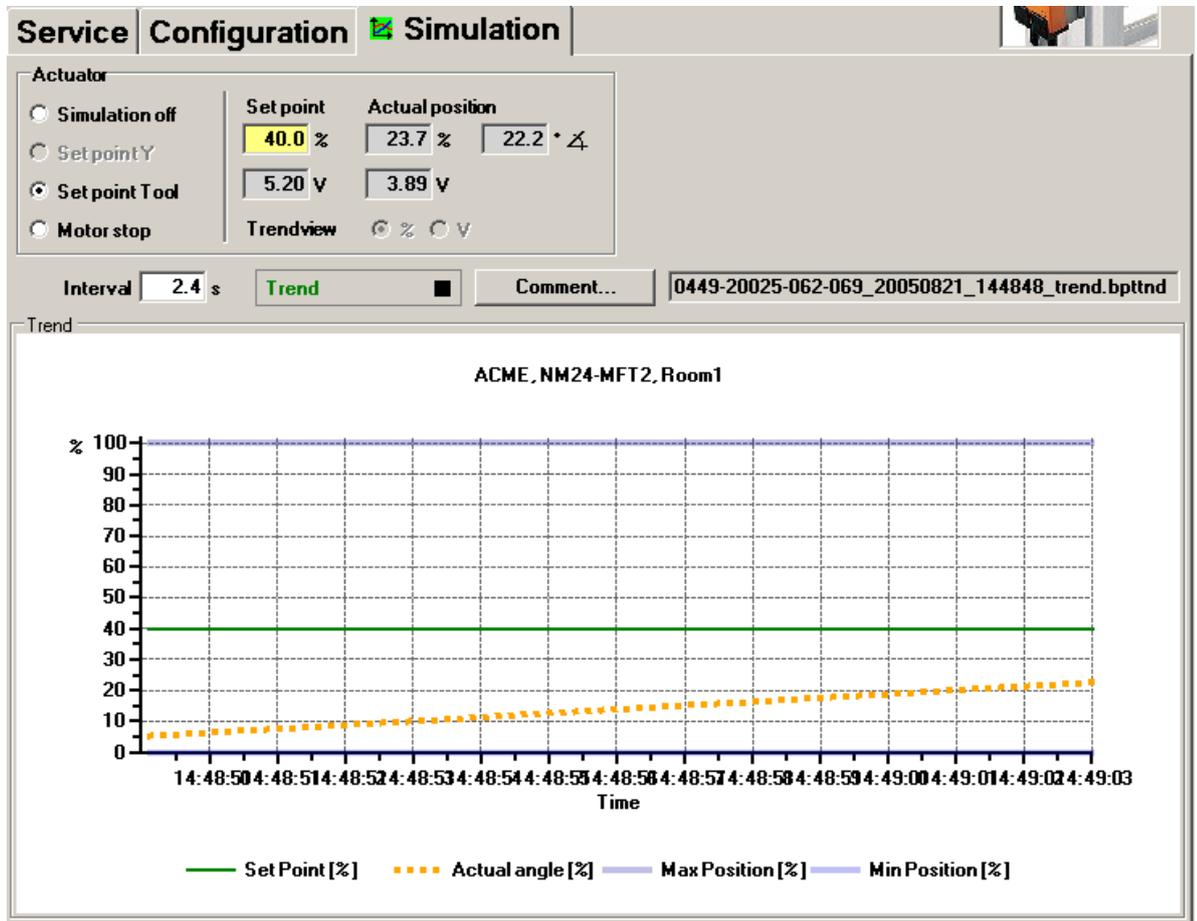
Simulation tab for damper actuators
