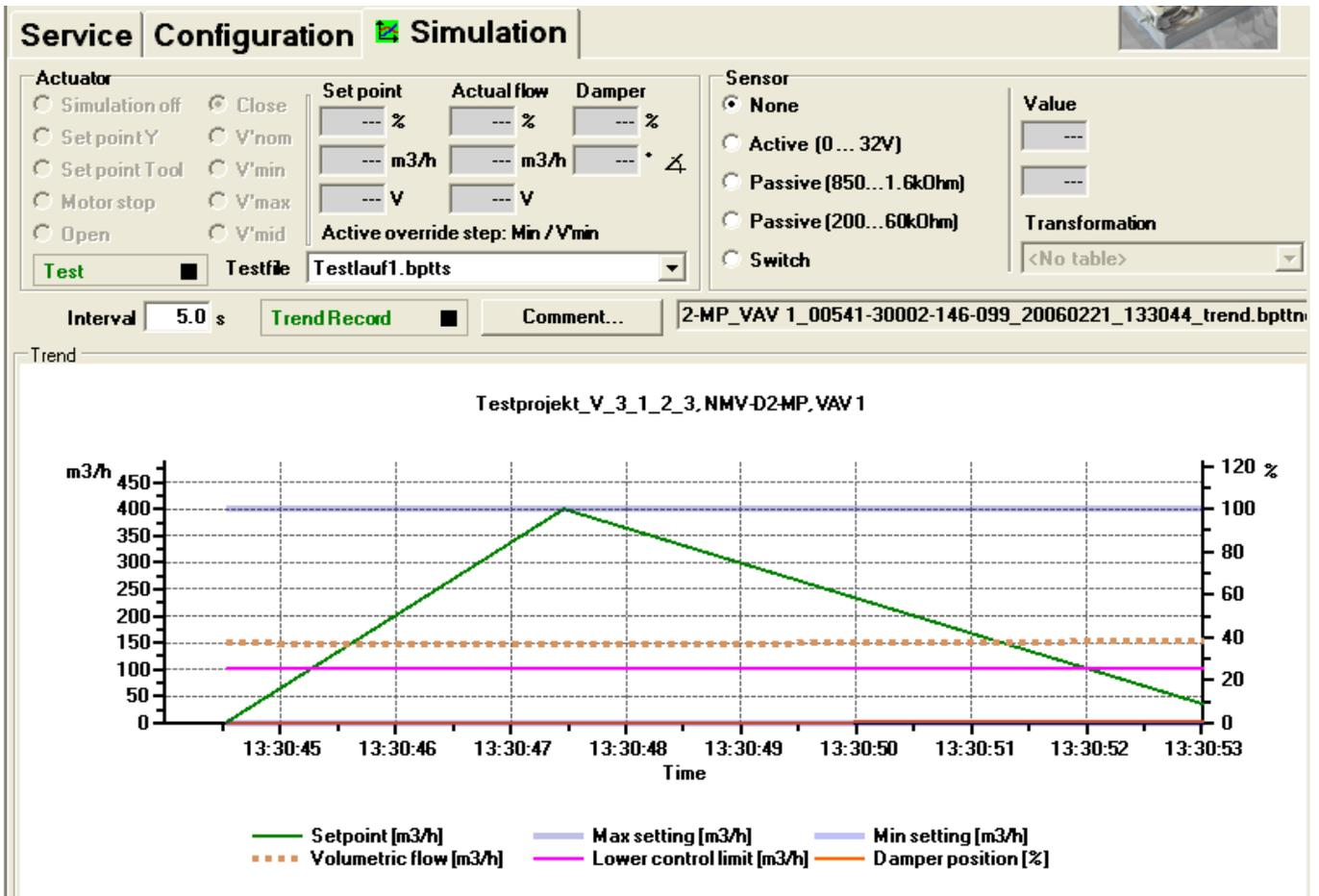
"Simulation" tab for VAV controllers
