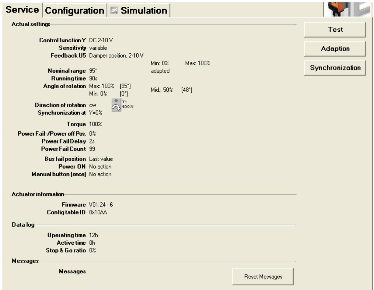
Service tab for full-rotation damper actuators
