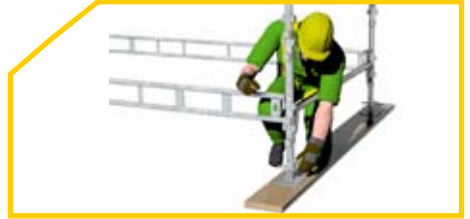
6 Connect all ledger and single beams to create a self standing frame.
