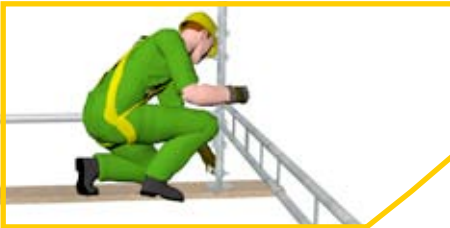
7 Using a spirit level adjust the jacks as required in a clock wise direction
