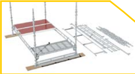
9 Select the appropriate equipment for subsequent lifts.
