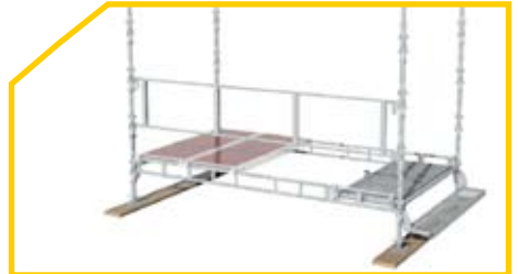
10 Fit Guardrail frame to guard 1st level Landing.
