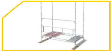
12 Ensure that sufficient standards extend 1m beyond the next lift and install Single Guardrail.
