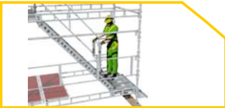
25 Fit Folding Guardrail Frame to protect lower Landing.
