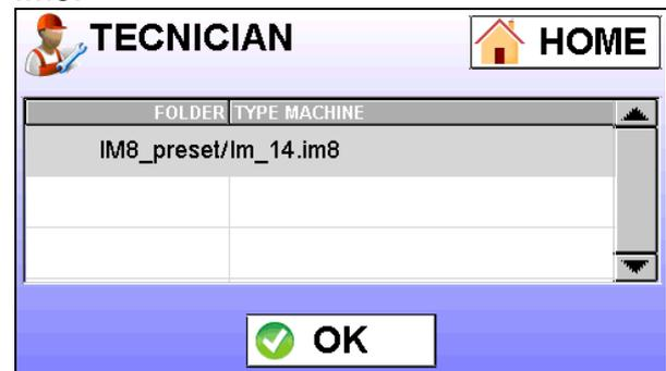
Select the desired preset machine and confirm with OK.
