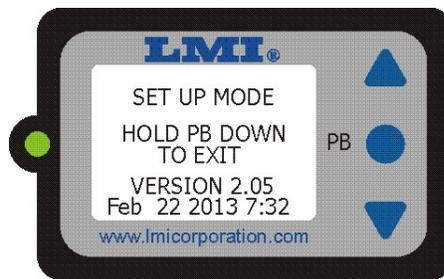
Press and hold the “PB” button for 3 seconds to return the gage to the main testing screen, which will also save any changes made to memory.
