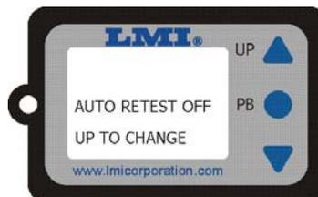
To change the setting, press the “UP” button, then press the “PB” button to save the changes and return to the main testing window.
