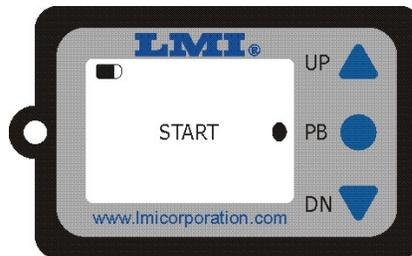
The unit will spend about 1 second determining its orientation and waiting for motion to stop. The green LED will come on and "WAIT" will be displayed on the screen, followed by "READY" displayed when the gage is ready to take a reading.
