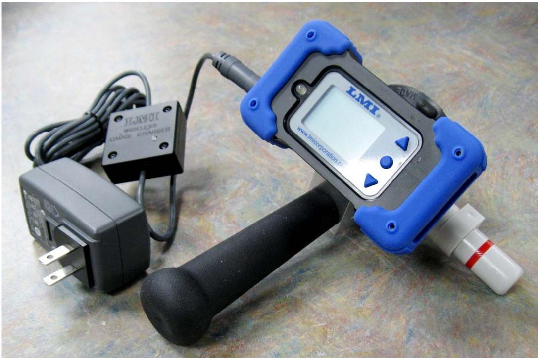
**Note:** The SK5477 G-Whiz Gage does not have an On/Off button. The gage will go into a low power “sleep” mode after 5 minutes of no activity, but will continue to draw a minimal current. Due to this low current draw, gages not used for a period of time or not left on a charger when not in use, will draw the battery down & require a full charge before being used.
