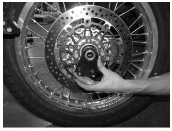
To re-install the wheel first place the caliper mount into the wheel.
