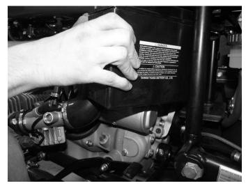
**Step 5**Carefully slide the battery out between the frame tube and air box.
