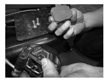
**Step 4**Remove the brake pads by pulling them out of
