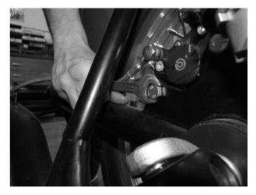
**Step 1**Remove the caliper mounting bolts.
