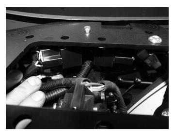
The relays are mounted to the frame base plate as shown.
