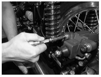
**Step 11**Re-install the brake caliper and brake pads.
