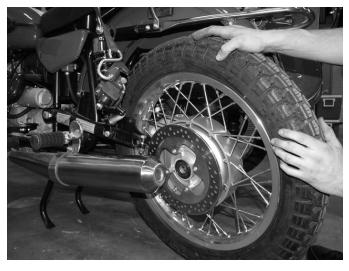
Remove the rear wheel by tilting the outwards towards you and rolling it back as shown.
