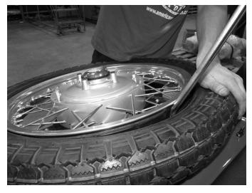
Using the provided tire spoons in your tool kit carefully remove one side of the tire from the
