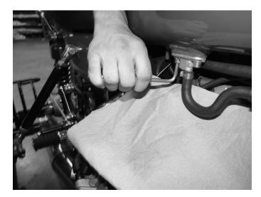
**Step 6**Remove the in-tank screen filter.
