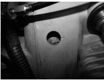
Remove the timing plug located on the right side of the engine case. Slowly rotate the engine using the kick start lever until both valves are closed and the TDC (top dead center) mark located on the flywheel is centered in the window.
