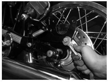
Remove the brake caliper mounting bracket bolts. Swing the support brace bracket up.
