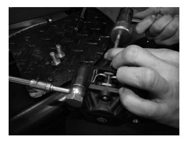
**Step 3**Remove the caliper safety clip and carefully drive the retaining pin out of the caliper with a punch or drift.
