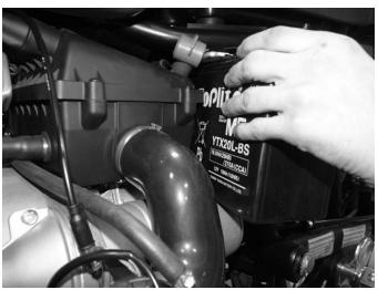
Re-install in reverse order by sliding the battery back into place and reconnecting all straps and cables.
