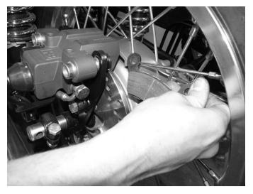
**Step 3**Remove the brake pads by pulling to the rear of the motorcycle.
