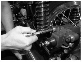
**Step 2**Remove the caliper retaining bolts.
