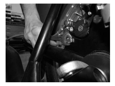
**Step 1**Remove the sidecar brake caliper.
