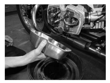
**Step 1**Starting with the left side cylinder, remove the valve cover and clean any contaminates found inside with a shop towel.
