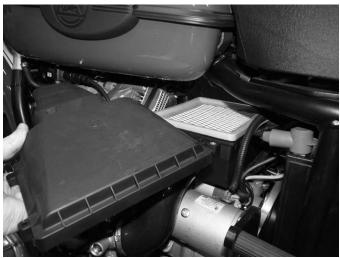
**Step 2**Carefully remove the air box lid by lifting the right side and sliding the lid to the left, be very careful not to pull wiring and cables near the
