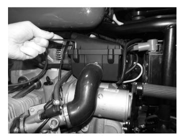
**Step 1**Remove the four retaining bolts form the air box lid using a 5mm hex wrench.
