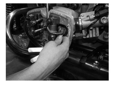
**Step 3**Using a feeler gage check the free play on both valves to confirm they are within specifications.
