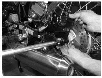
**Step 9**To re-install the rear wheel place the wheel back on the bike and push the axle through both the wheel and brake mounting bracket as shown.
