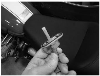
Clean all debris for the intake filter and re-install in the tank.
