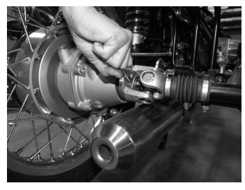
**Step 6**Remove the rear axle nut.
