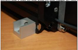
1. Insert the t-nut in the end of the stage as shown and slide it to the desired position.
