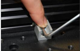
3. Use M6 or 1/4"-20 screws to mount the brackets to a mounting surface.
