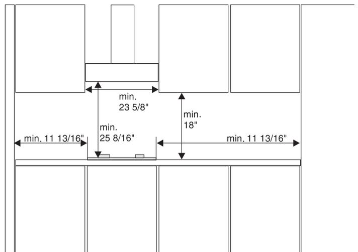
If several cook tops are installed next to each other, please observe the minimum distances between the cuts into the counter top as indicated in the drawing.
