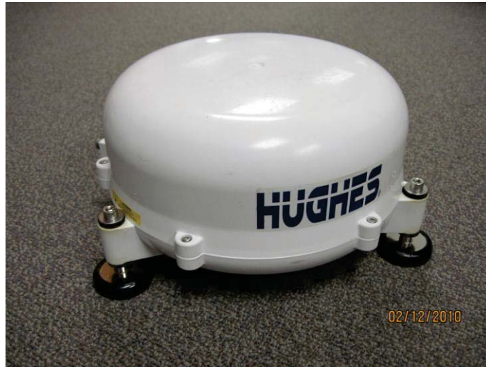
Figure 13 – C11 Antenna ODU Ø252 mm x 119 mm Height
