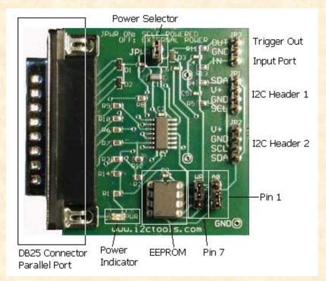
**DB-25 Parallel Port Connector** - plugs into the computer's printer (LPT) port.
