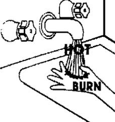
The temperature-pressure relief valve must be manually operated at least once a year. Caution should be taken to ensure that (1) no one is in front of or around the outlet of the temperature-pressure relief valve discharge line, and (2) the water manually discharged will not cause any bodily injury or property damage because the water may be extremely hot.
