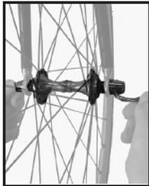
Figure 3- Wheel quick-release
