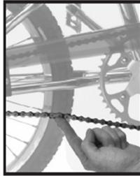
Figure 6- Checking chain tension
