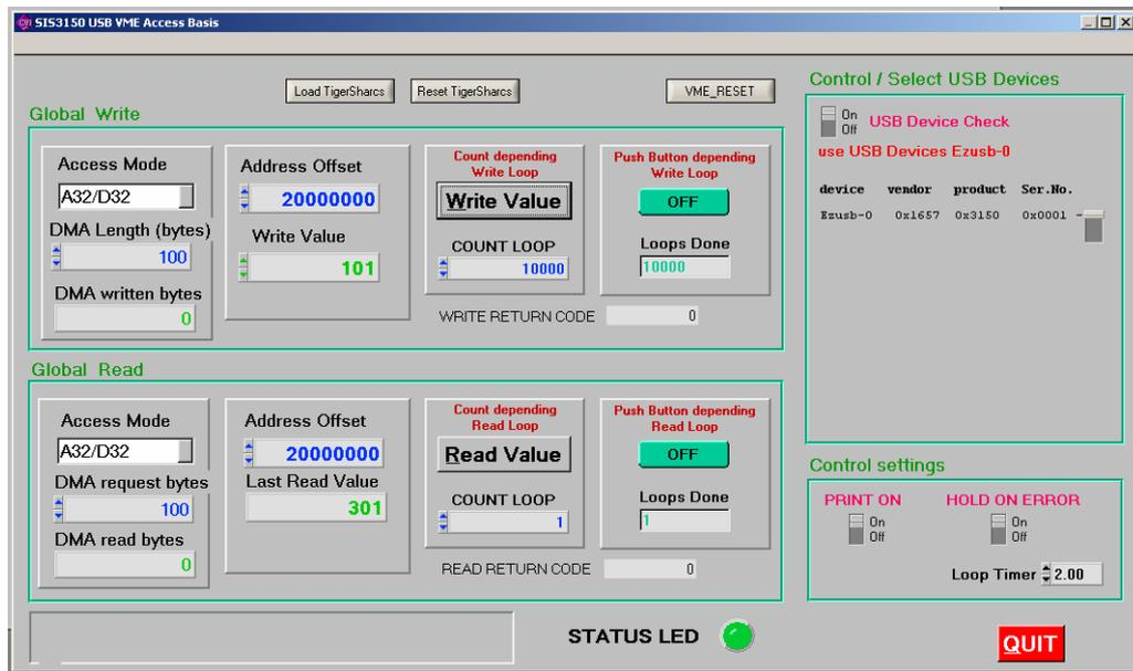
**Note:** The SIS3150 USB base program checks for USB devices in a cyclic manner as long as the USB Device check slide bar is set to On. The scan resets the user LED on the SIS3150 in case it was set/switched on with a control write.
