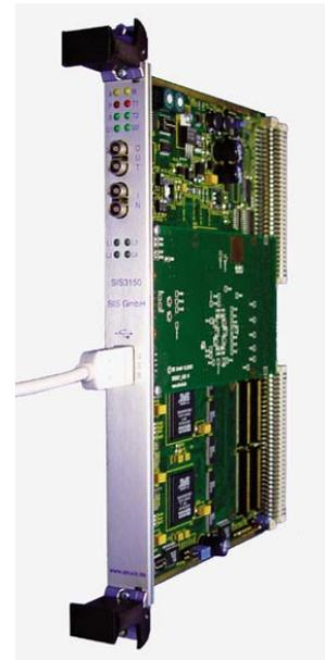
The use of the 2<sup>nd</sup> CMC site of the SIS3150 for a frontend card like the SIS9300 4 channel 100 MHz 14-bit digitizer board allows you to build efficient systems with and without making use of the VME bus. A 4 channel ADC/digitizer system of that type in a rackmount box is shown below.
