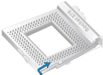
2. Align the blunt edge of the CPU with the matching pinhole distinctive edge on the socket.
