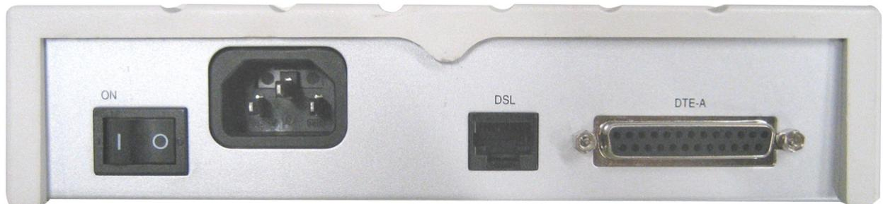
Figure 5 The ***I-DSL128*** rear panel
