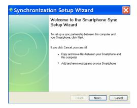
At subsequent ActiveSync sessions, press **Cancel** to be able to exchange files between your handset and your PC via the Explore function. Do NOT press **Next** at this stage unless you wish to access advanced functions.
