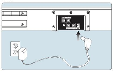
Plug the small end of the power cord into the DC Input on the back of the speaker, and the large plug into a standard wall outlet.
