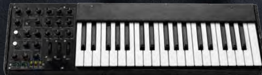
2-oscillator, monophonic analog synthesizer by Hans Nordelius, 1976.
