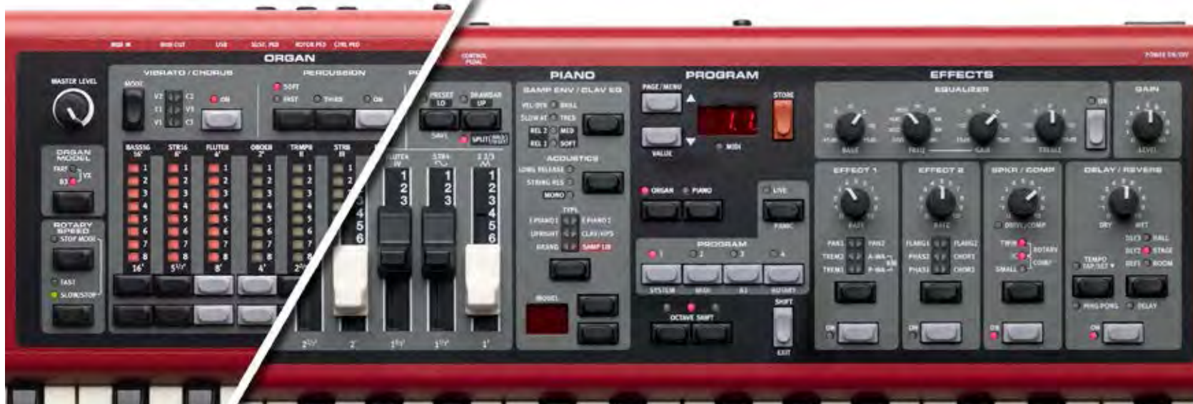
The Nord Electro 4 SW73 and Nord Electro 4 HP features our Digital LED drawbars while the Nord Electro 4D features physical drawbars.
