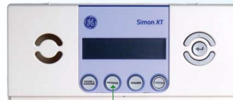
**Tip:** Stay Mode refers to arming only your monitored doors and windows. You can also arm just your Motion Sensors by pressing only the Motion button. This can be useful if your sensors are located in a basement or a different area of the home where you rarely go. Keep in mind that arming the Motion Sensors when people are in the house increases the likelihood of a false alarm.
