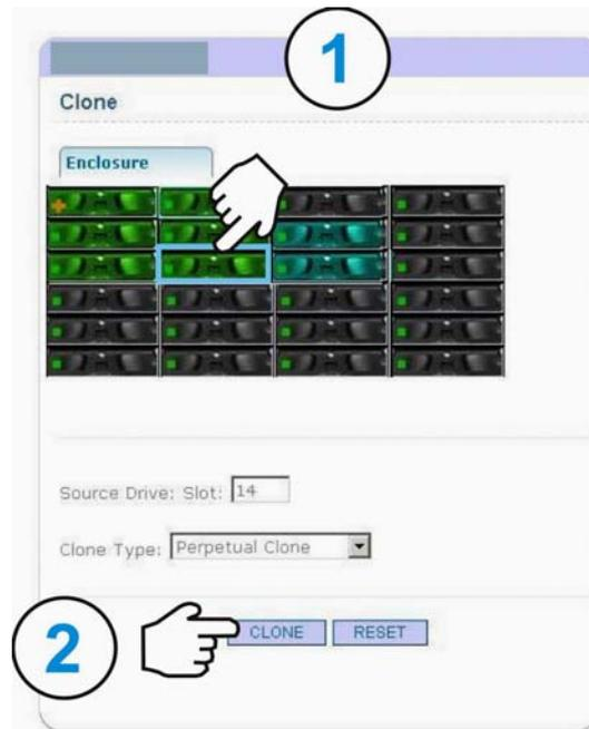
Figure 4-9: Cloning a Target Drive
