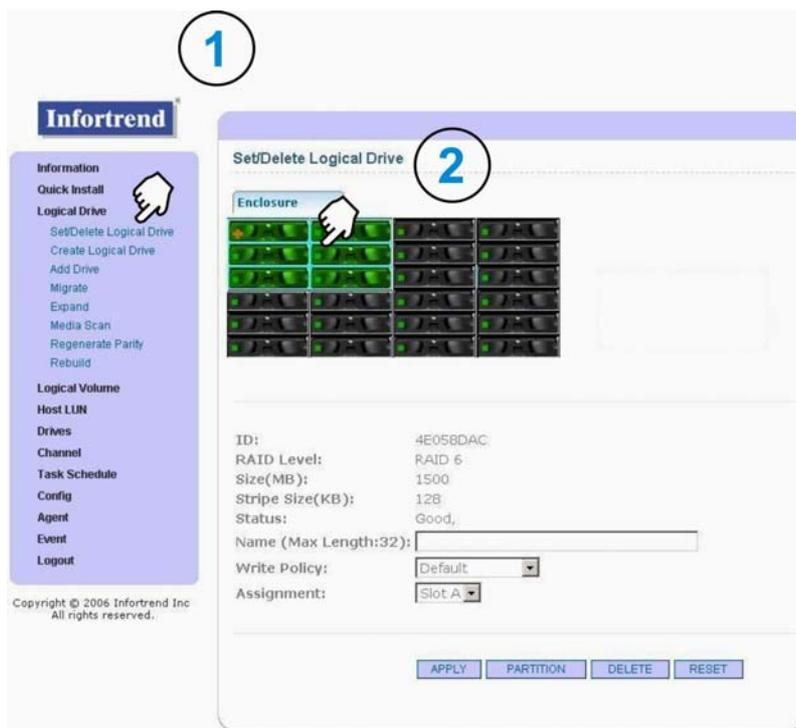
**Figure 3-6: Configuring Logical Drive Parameters**
