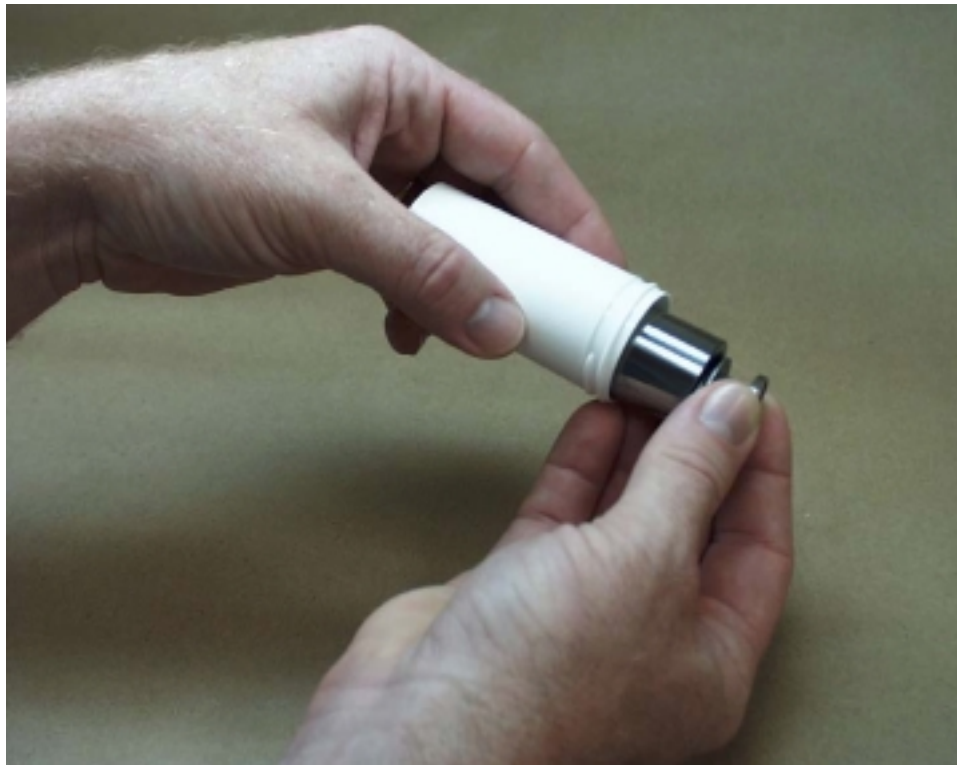
FIGURE 5-3 REMOVING LOW RANGE PISTON AND CYLINDER FROM CONTAINER
