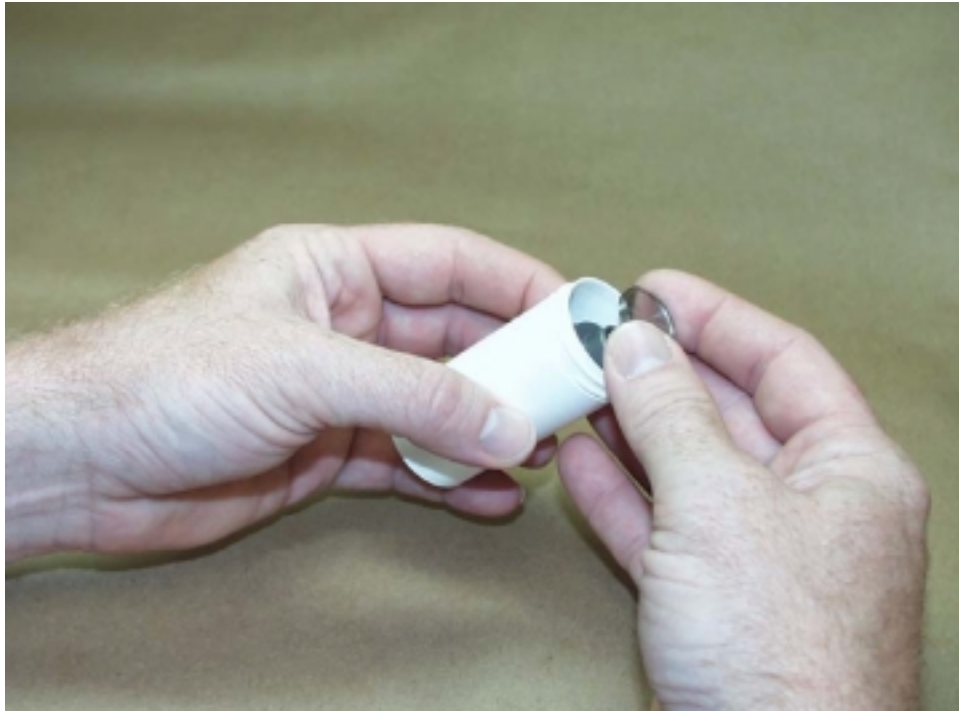
REMOVING LOW RANGE PISTON AND CYLINDER FROM CONTAINER
