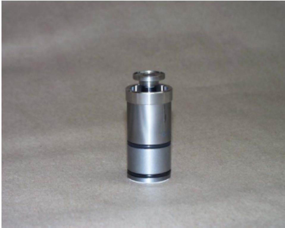
FIGURE 5-8 MID RANGE PISTON/CYLINDER ASSEMBLY
