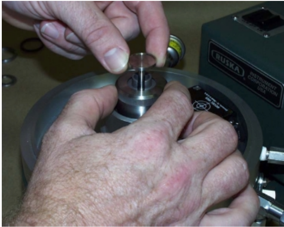
FIGURE 5-6 POSITIONING THE UPPER THRUST WASHER/PISTON RETAINER IN THE CYLINDER RETAINING CAP RECESS
