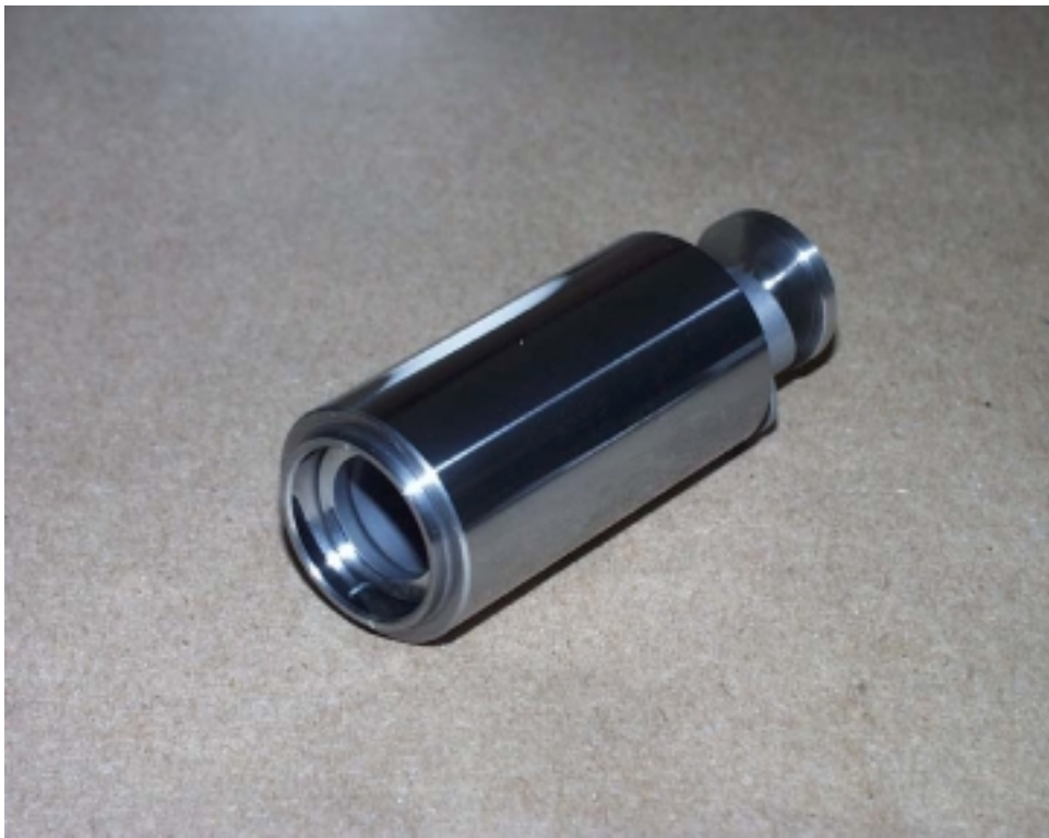
FIGURE 5-5 LOW RANGE PISTON AND CYLINDER SHOWING O-RING GROOVE
