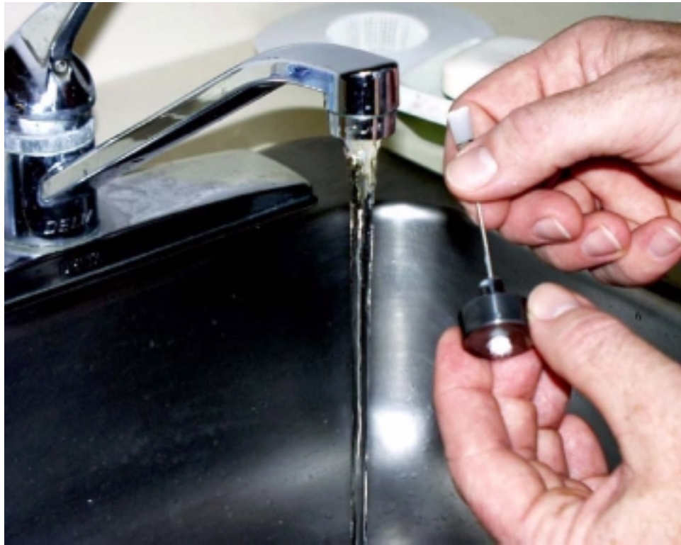
FIGURE 6-13 CLEANING THE HIGH RANGE CYLINDER
