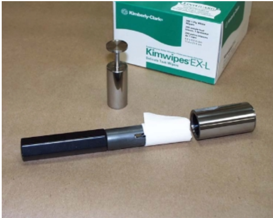
FIGURE 6-6 PREPARATIONS THE LOW RANGE CLEANING TOOL
