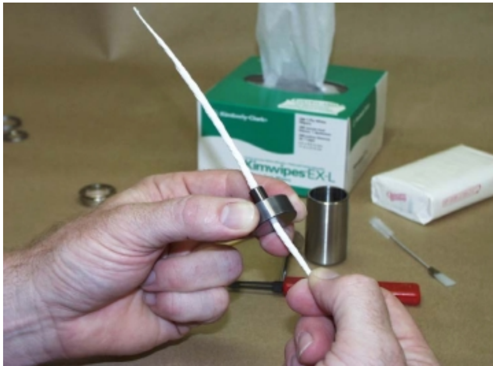
FIGURE 6-14 DRYING THE HIGH RANGE CYLINDER
