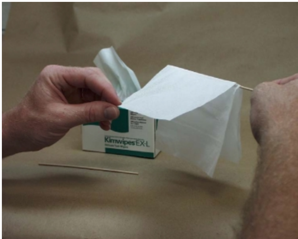
FIGURE 6-2 PREPARATIONS FOR CLEANING THE LOW RANGE CYLINDER
