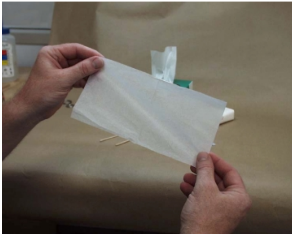
FIGURE 6-10 PREPARING KIM WIPE FOR CLEANING THE HIGH RANGE CYLINDER
