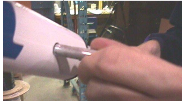
Clip the locking clip back onto the clevis pin.
