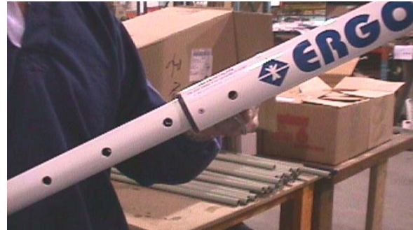
Insert the clevis pin back in into the boom.
