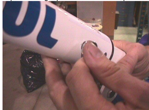
Clip the locking clip back onto the clevis pin.
