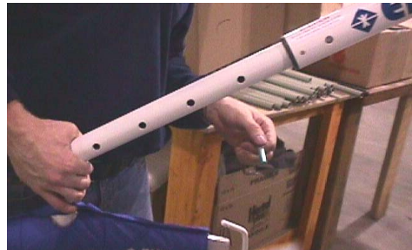
Align the hole of the boom and the extension.
