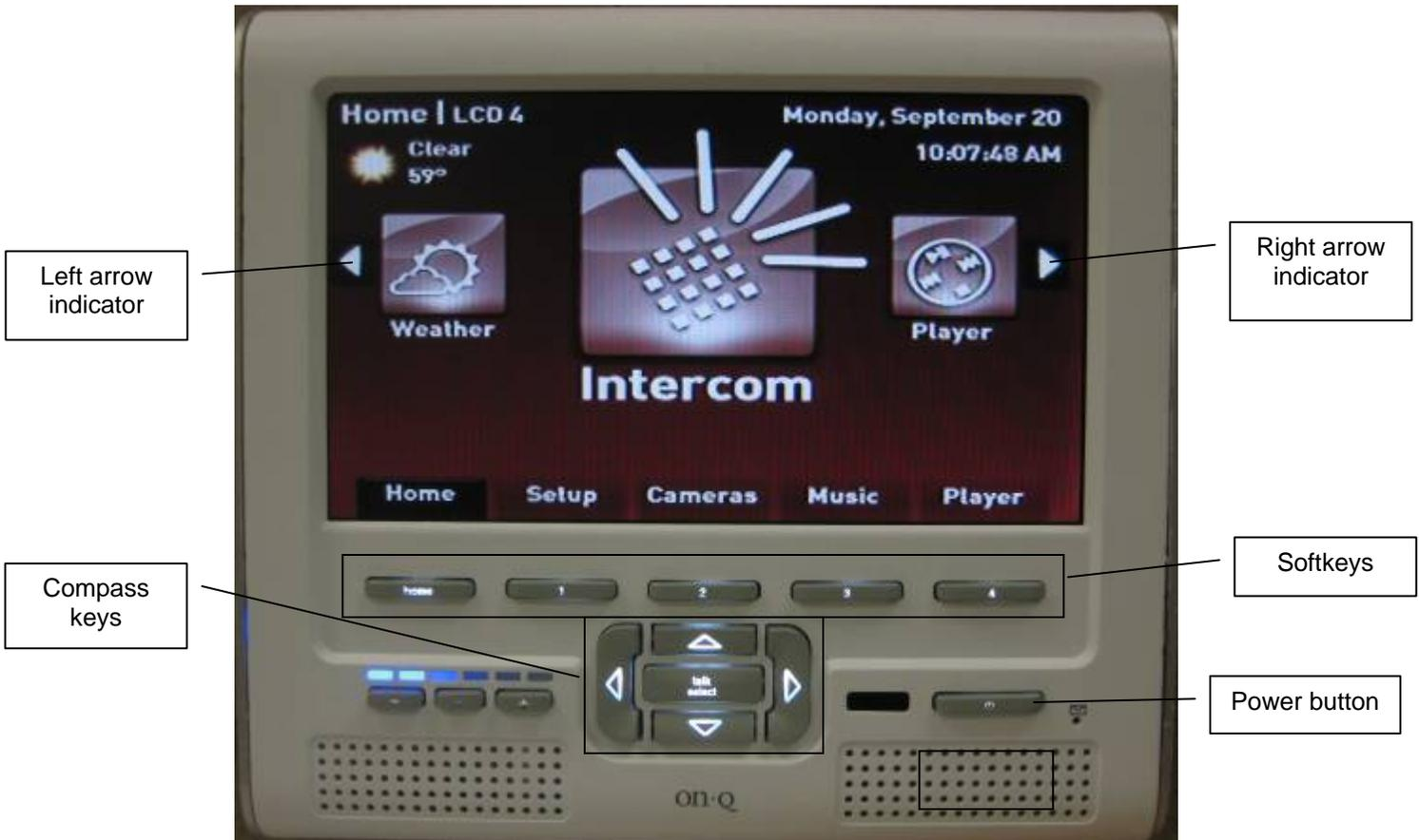
Above is a description of the various buttons on the front of the Unity LCD Console. Each softkey corresponds to the tab shown directly above it in the display. Similarly, the compass keys correspond to the associated arrow indicators shown in the display. For instance, in this particular screen, the left and right compass keys would move the Icon Wheel to the left or right accordingly.
