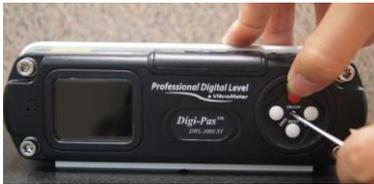
Ensure the DWL3000XY device is in power OFF condition. Press and hold the CAL button by using a small pin and simultaneously press the ON/OFF button. The LCD screen displays “Calibration 1”.
