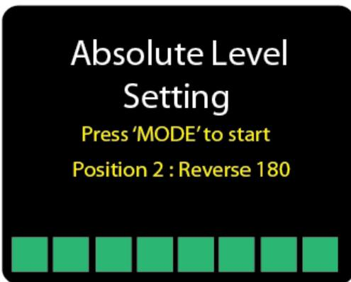
Turn the device 180° and press MODE button again to start the measurement.
