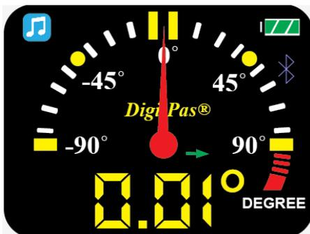
Once Bluetooth mode is activated, the icon
