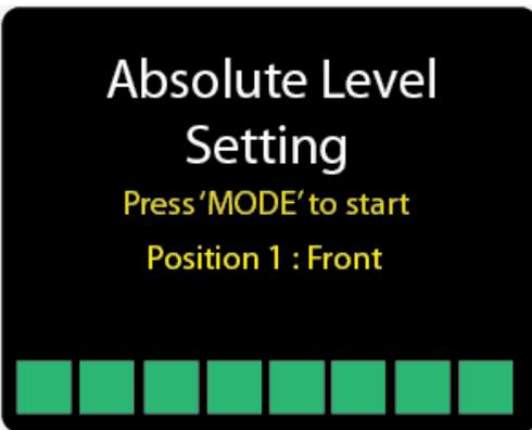
Place the device on the surface to be measured. Press MODE button to start the measurement and wait until the loading bar is full.
