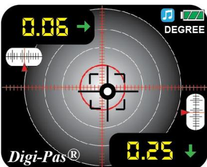
Once the measurement stabilizes, the “Target Ball” or “Bull Eye” blinks.
