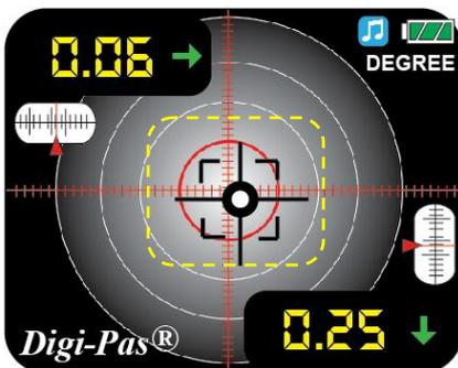
The “Target Ball” or “Bull Eye” move towards the measured position similar to traditional "Bubble" vials. The green arrow sign on display indicates the higher side of plane.
