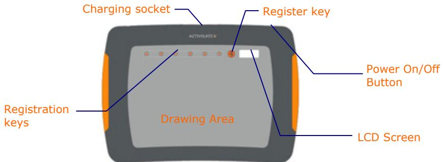
The Activslate is supplied with a partially charged battery. You are advised to charge the battery completely before using the Activslate. Insert the connector from the power supply cable into the Activslate charging socket, then plug into the mains supply and apply power. The Activslate will take approximately 3 hours to charge.
