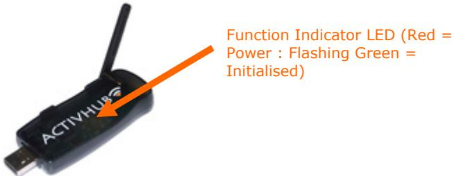
When the driver has been detected, the red Function Indicator LED changes to flashing green, this indicates that the device has initialised.
