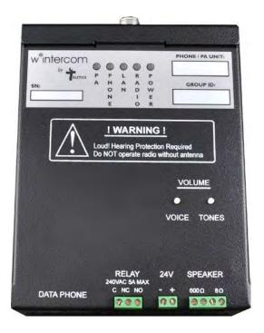
**Phone** indicates that the phone attached to the wintercom unit has gone "off hook". This shows you that the phone is correctly attached to the wintercom unit.
