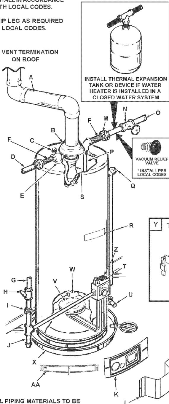
INSTALL THERMAL EXPANSION TANK OR DEVICE IF WATER HEATER IS INSTALLED IN A CLOSED WATER SYSTEM
