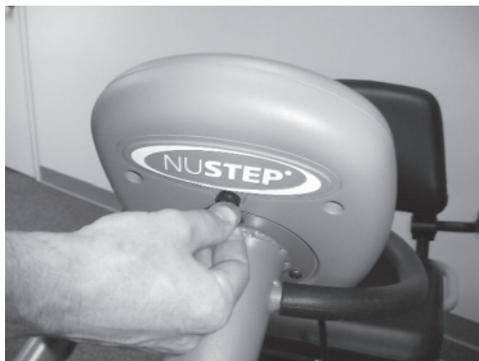
2. Replace the 4 AA alkaline batteries. (NiMH rechargeable batteries may also be used.)
