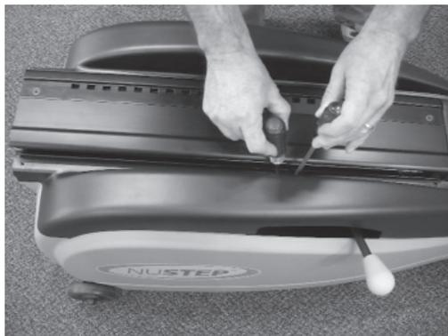
For top cover installation, place scratch awl in third hole from front to align holes, then insert 3 screws. Repeat for opposite side.
