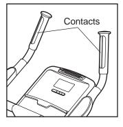
rate, hold the handgrip pulse sensor with your palms resting against the metal contacts. Avoid moving your hands or gripping the contacts tightly.
