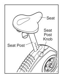
**adjustment holes in the seat post.** Then, turn the knob clockwise to tighten it.
