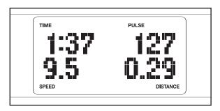
The lower left corner of the display will show your pedaling speed, in miles or kilometers per hour.
