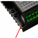
Figure 5. Grounding Screw on the Chassis
