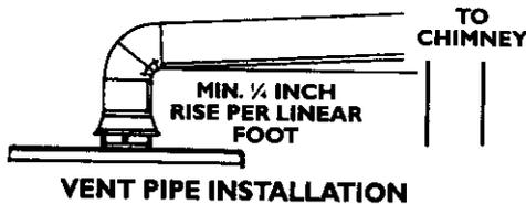
There must be a minimum of 6" clearance between single wall vent pipe and any combustible material. Fill and seal any clearance between single wall vent pipe and combustible material with mortar mix, cement, or other noncombustible substance. For other than single wall, follow vent pipe manufacturer's clearance specifications. To insure a tight fit of the vent pipe in a brick chimney, seal around the vent pipe with mortar mix cement.
